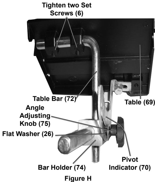
2. Insert free end of Table Bar into two Mounting Supports on bottom of Table. Tighten the two Set Screws (6). Refer to Figure H.
